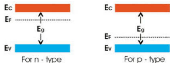
Figure 3.2: Fermi Level in Extrinsic semiconductors
