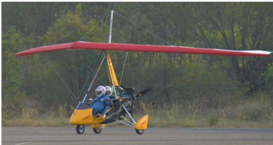
Cruiser powered Hang Glider with Rotax 582 Engine and Aeros Stil 17 Wing
