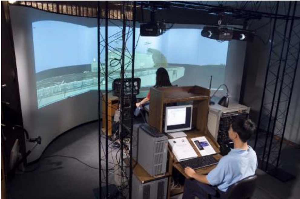
Flight simulator with pilot in front of projection screen and operator at rear console
