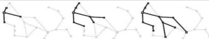
Figure 3.8 A sequence of search trees generated by a graph search on the Romania problem of Figure 3.2. At each stage, we have extended each path by one step. Notice that at the third stage, the northernmost city (Oradea) has become a dead end: both of its successors are already explored via other paths.
