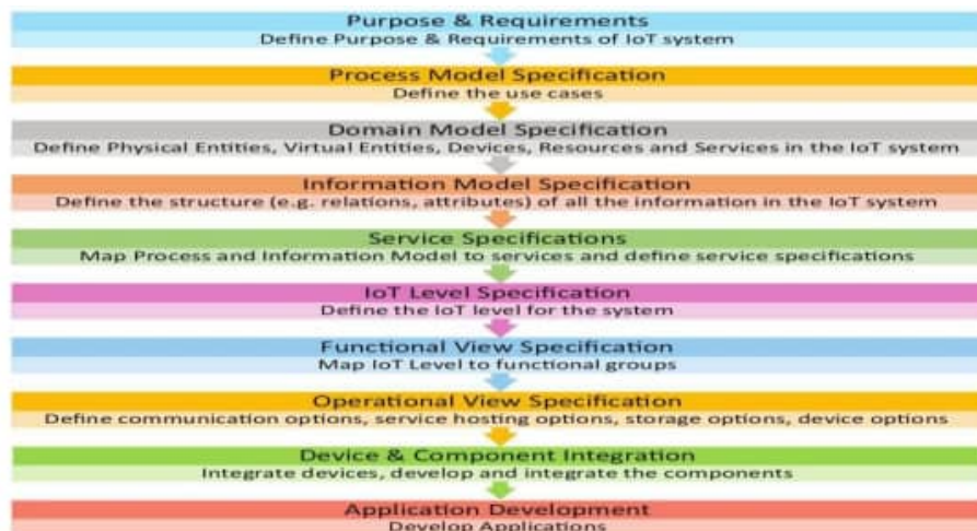
Figure 3.1: Steps involved in IoT system design methodology
