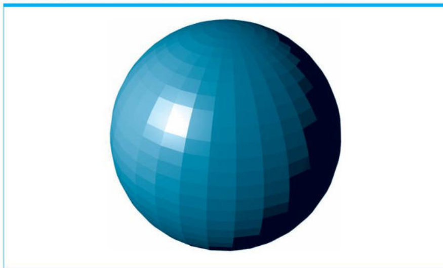
Figure 10.10 A sphere as it might appear when rendered by flat shading
