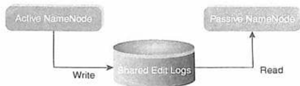
Figure 5.26 Active and Passive NameNode interaction.
