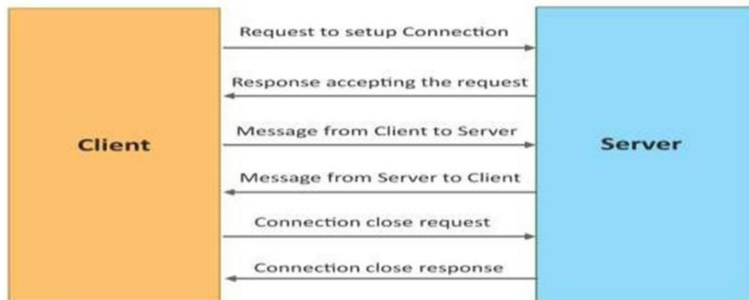
Figure 1.8: block diagram of Exclusive Pair Communication Model
